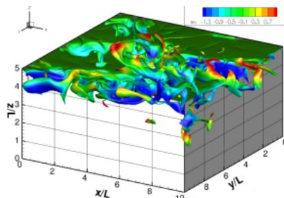
Simulation result: isosurface of 50% concentration saturation ( $Sc = 20$ )
