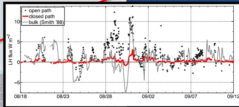
Water vapor cross-sensitivity can be a significant challenge for EC  $\text{CO}_2$
