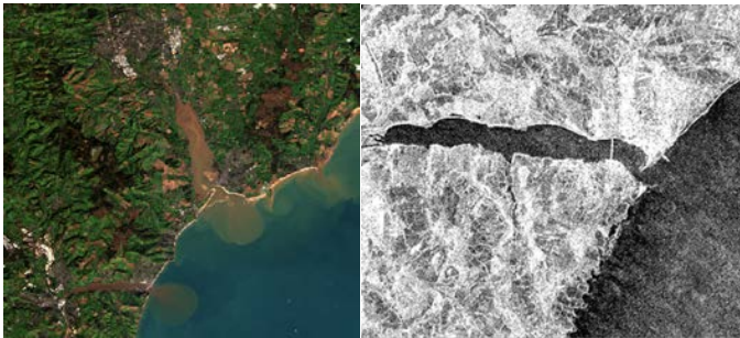
River plumes in East Devon (left: Exe and Teign, Landsat8 pseudo-true colour composite; right: Teign, a Sentinel-1 SAR backscattering image).
